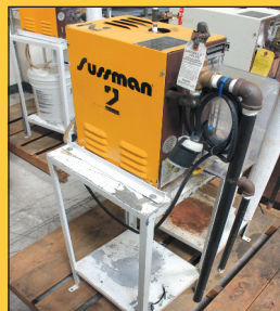
Sussman Steam Generator
